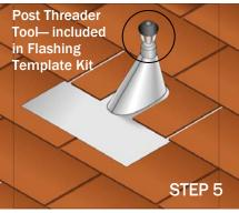
STEP 5: Using the post threader tool (included with the flashing template), thread the post through the flashing into the base.
