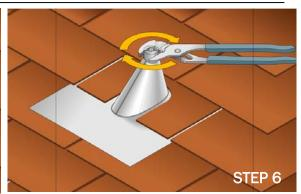
**STEP 6:** Using the adjustable pipe pliers, tighten post into base by turning clockwise.
