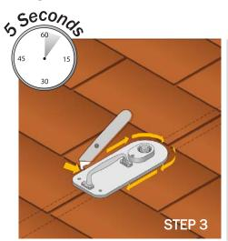
STEP 3: Using a FastJack® flashing template (optional), and a utility knife with hook blade, cut composition shingle. The template will cut the shingle to the size needed for a standard or Oatey® flashing. (TEMP-STD illustrated)
