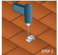
STEP 1: Locate rafter center by using precision stud finder or other means. Using a 3/8" masonry bit, break through the comp shingle over the rafter in the center of the shingle. Position Fast-Jack® drill guide over the hole location and drill your pilot hole using a 3/16" drill bit.
