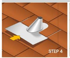
**STEP 4:** Slide flashing over the base and under the upper row of composition shingle.
