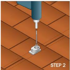
STEP 2: Insert the 5/16" stainless steel lag bolt and washer through the FastJack® base. Install the lag bolt through the FastJack® using a ½" socket and electric impact wrench.
